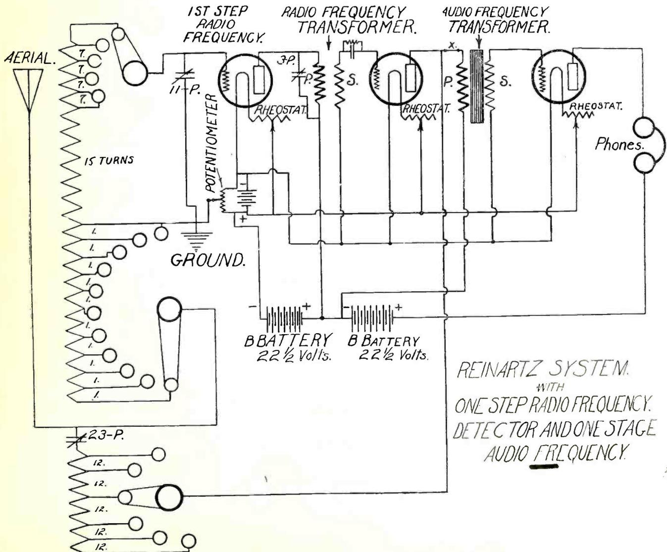
radio frequency. They are then carried to the detector tube, where they are rectified and brought down to audio frequency. From this it will be seen that radio frequency amplification will really magnify oscillations received upon the aerial and pass them to the detector tube for rectification.
